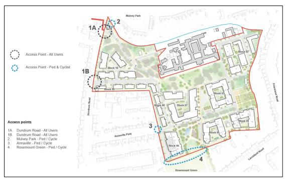
Figure 4.4: Extract from Reddy A + U *Architectural Design Report* showing proposed access points and breaks in the perimeter wall.
